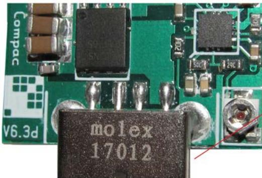
Approximate position of potentiometer on stock units. Notice flat part of screw head, and use it as your reference point.
